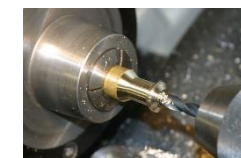
Figure 1: the collet chuck allows material to be gripped without damaging the outside surface.
